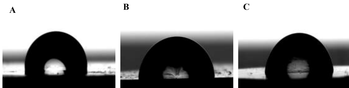
Figure 3.5 Water contact angle for A) sPS B) PI and C) PUA compressed aerogel disk
