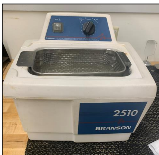
Figure 22: The ultrasonic device for clean the current collectors (Branson 2510).
