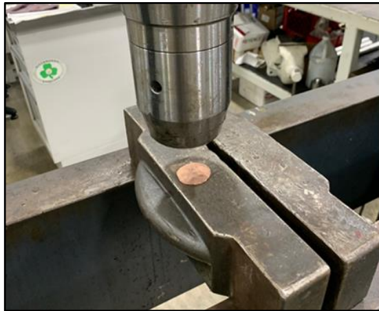
Figure 15: press for forming the samples (DAKE -50 Tone).
