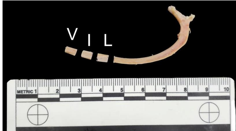
Figure 25. Representative image of serial sections procured from each rib, Ventral (V), Intermediate (I), and Lateral (L), in preparation for compression testing. Apparent differences in shape are due to resting orientation of sections in the image.
