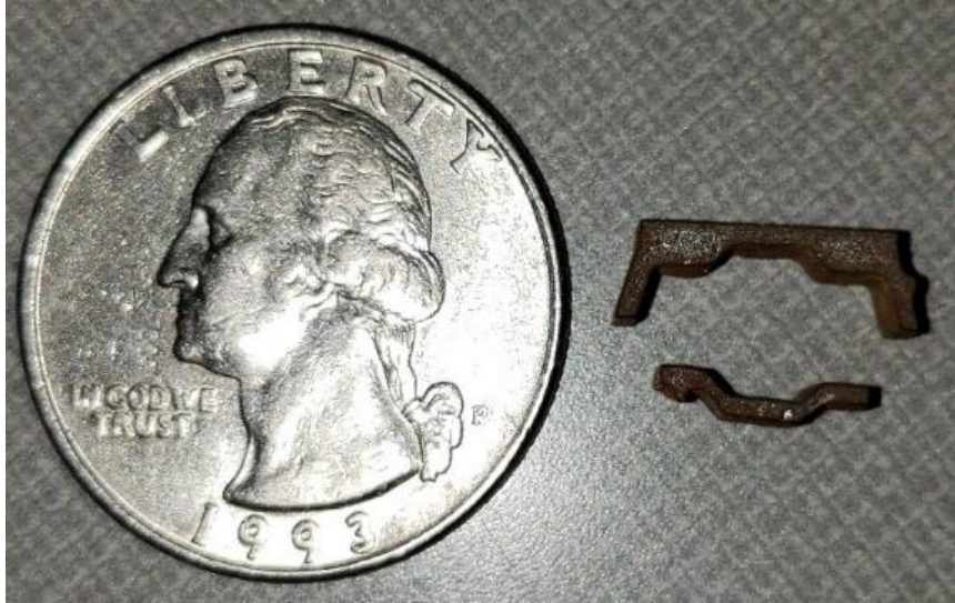
Figure 8. Top and bottom layers of the PEH manufactured from low carbon steel by the use of the waterjet cutting method.
