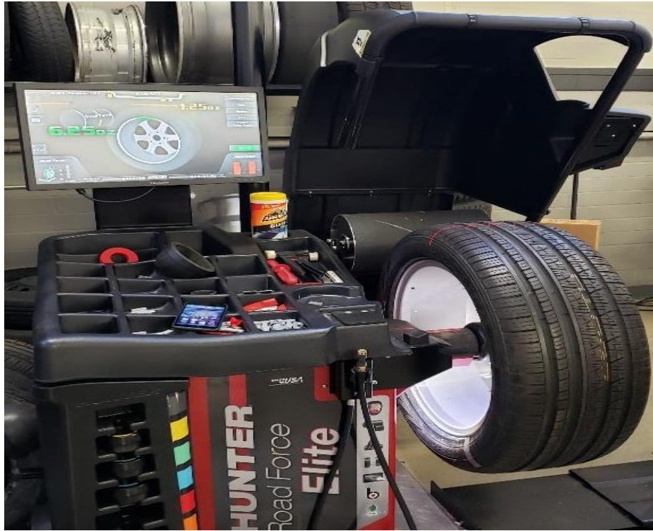
Figure 11. The experimental setup. The tire setup on the Road Force Elite machine [109].
