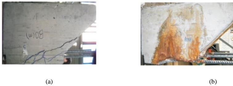
Figure 3.4 Different failure modes observed by Hanjari et al. (2011): (a) pull-out failure, (b) splitting failure
