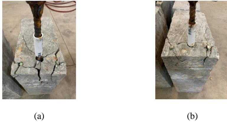
Figure 2.6 A typical cracking pattern for (a) splitting failure mode and (b) pull-out failure mode.
