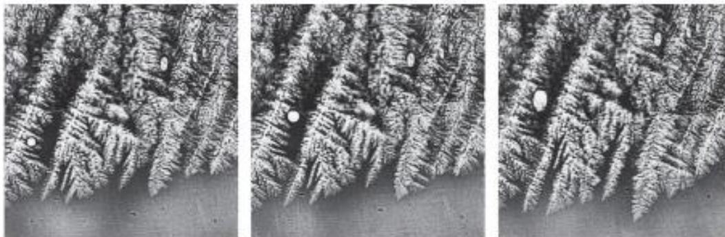
Figure 33. Gas porosity evolution in a directionally solidified Al-30 wt% Cu alloy. (Courtesy of R. Mathiesen, Sintef,[124]).
