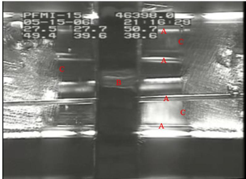
Figure 3. PFMI 15 experiment showing the heater moving towards the left, leading to solidification of the melt from the right.
