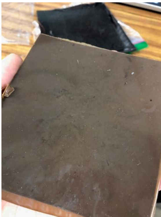
Figure 2-8. The compression molded glucose-NR composite at 1.25 phr.
