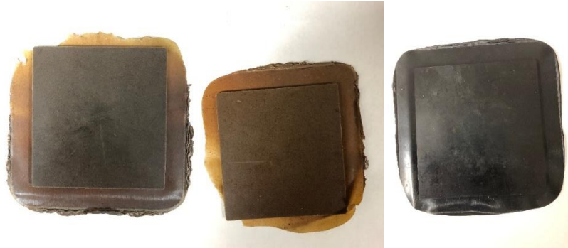
Figure 2-9. Rubber with Blended Hydrolysate (left), Sonicated Hydrolysate (middle), Carbon Black (right).
