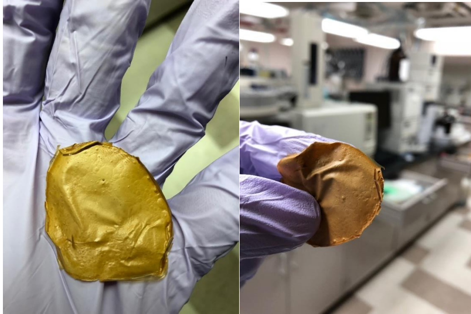
Figure 1-17. Film-like appearance of oven-dried filtrate ( < 2.7 \mu\text{m} ) after sonication.
