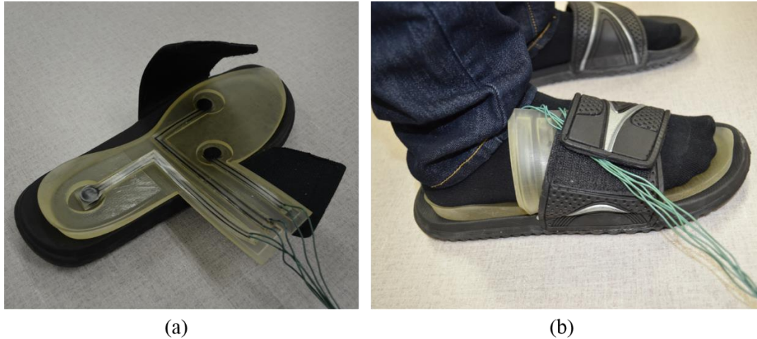
Figure 3.29. Insole with the wired sensors was put in a sandal: (a) electrical wires were pierced into sensor electrodes; (b) insole in sandal before walking [63].
