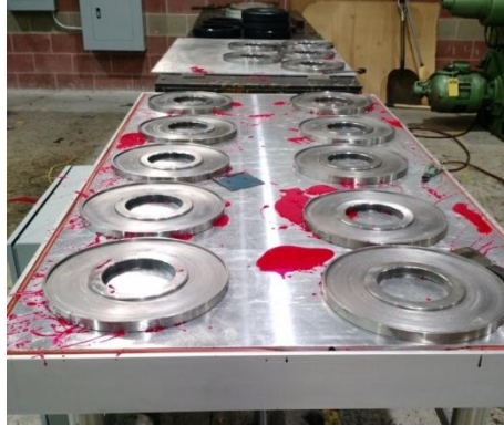
Figure A.1.11. Cast for Red Gasket Ring kept over the heated table
