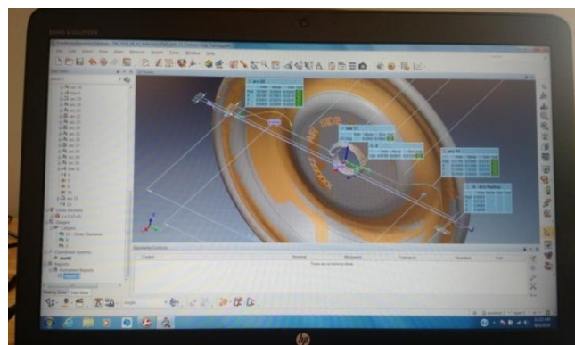
Figure A.1.34. Object (Data) fitted on the CAD model (Reference)
