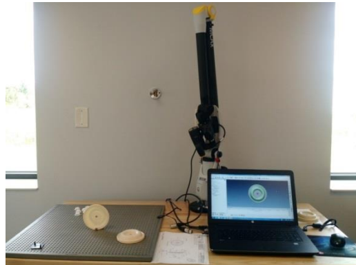
Figure A.1.12. 3D Scanner with Polyworks software running on the computer
