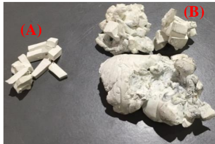
Figure A.1.14. (A) Small Pieces of the material that were fed to the machine. (B) Curled up material strips from the throat of the injection carriage.
