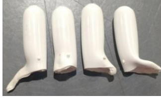
Figure A.1.19. Appearance of molded parts from 2018PFM-5Batch#1 without using a mold release agent
