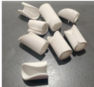
Figure A.1.20. Incomplete molded parts from 2018PFM-5Batch#1 due to low injection volume
