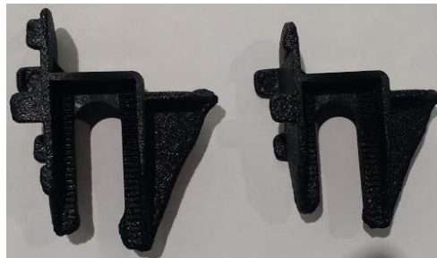
Figure A.1.28. Injection molded part with 500 psi injection pressure
