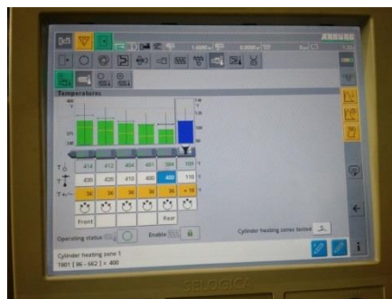
Figure A.1.17. Temperature conditions for molding 2018PFM-5Batch#1
