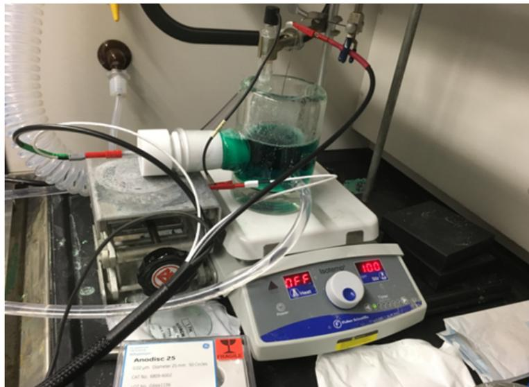
Figure 3.2: Photograph of three electrode electrodeposition technique
