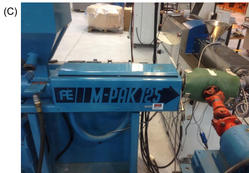
Figure 4-8 (A) Schematic illustrates the three different heating zones of the single screw extruder with a gear pump stabilizing output pressure; Photos of the extruder and gear pumps for (B) core-material (Rheomex 252P), (C) shell-material (Akron Extruder M-PAK 125)
