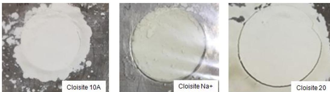
Figure 4.15 Photographs of nanoclay disks after thermal aging for 30 minutes at 180°C
