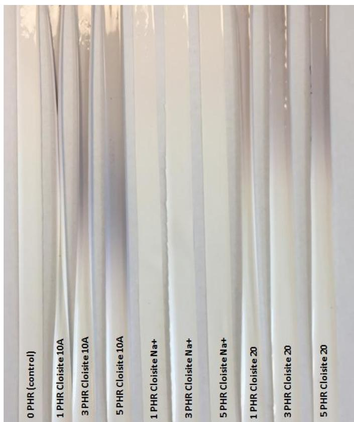
Figure 4.14 Photographs of the white films after heating in Metrastat
