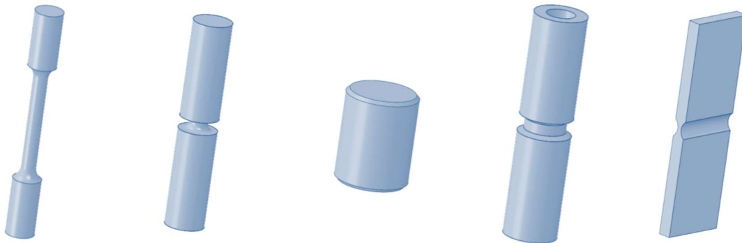
Figure 6.1. Sketches of a smooth round bar, a notched round bar, a compression specimen, a torsion tension specimen, and a flat grooved plane strain specimen.
