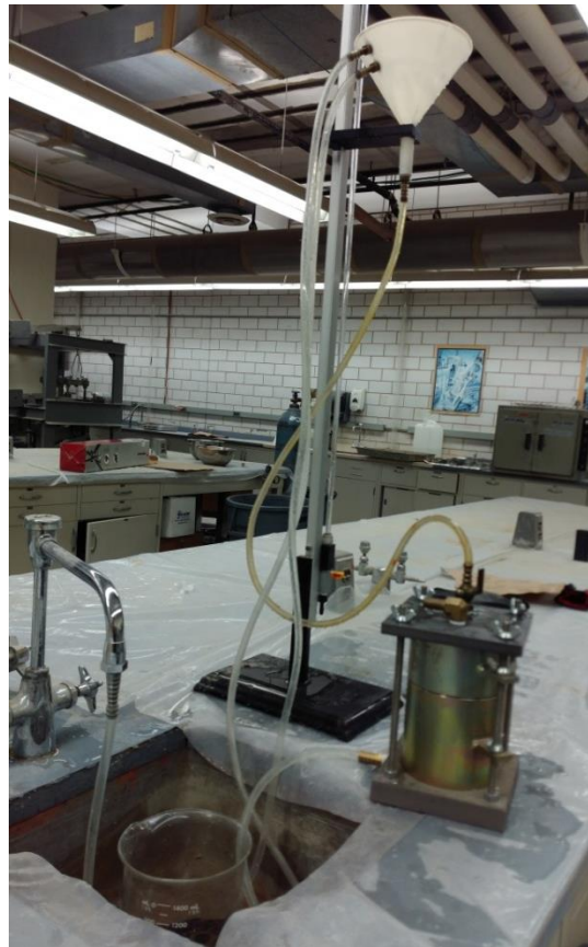
Figure 3-6: Permeability test setup
