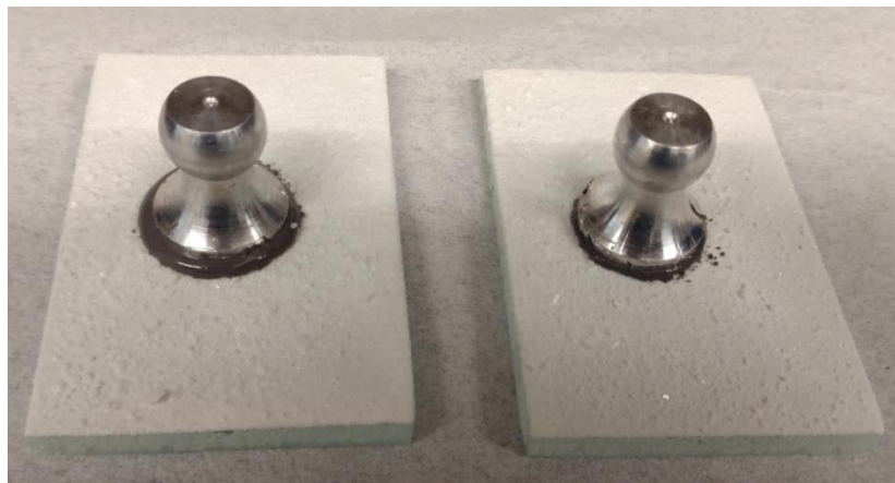
Figure 4-8: Sample preparation for pull out test
