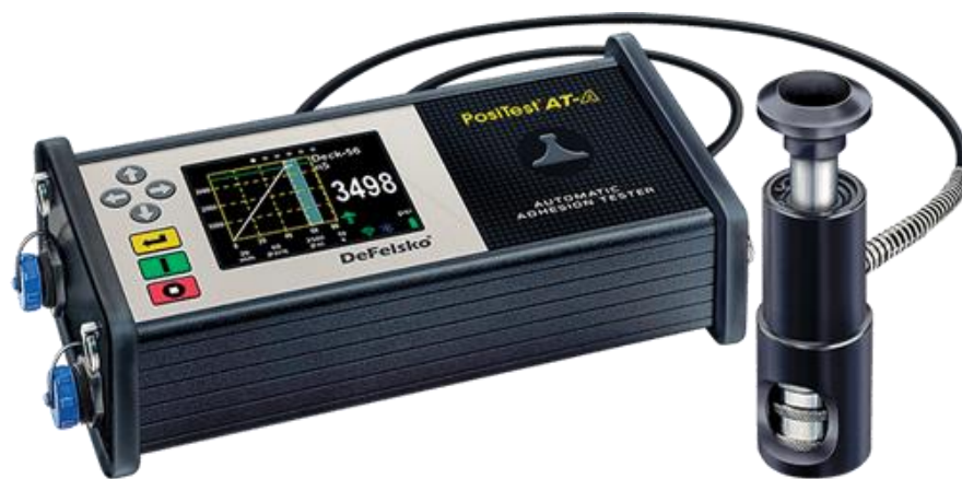
Figure 4-9: Pull out testing device to determine bond strength (Image source:[41])
