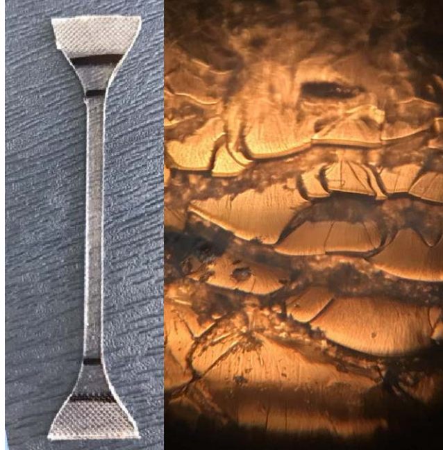
Figure 4.9 Photo of the dog-bone shaped specimen cutting from the hot-pressed film (left) and the side surface from microscope (right) perpendicular to the paper, with cutting direction from top to bottom. The specimen in the left is put under Carl Zeiss microscope with 10X eyepiece and 10X objective lens.
