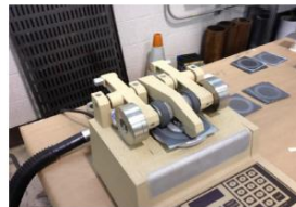
Figure 4.2: Taber Abrasion Apparatus
