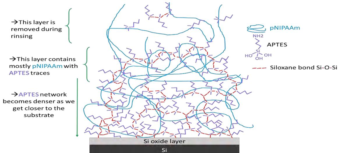
Figure 4.5 A schematic illustration of the network after the segregation of APTES in the pNIPAAm/APTES film during the curing processes.
