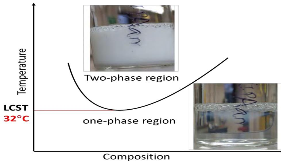
Figure 2.1 The phase separation of pNIPAAm/water solution above the LCST.
