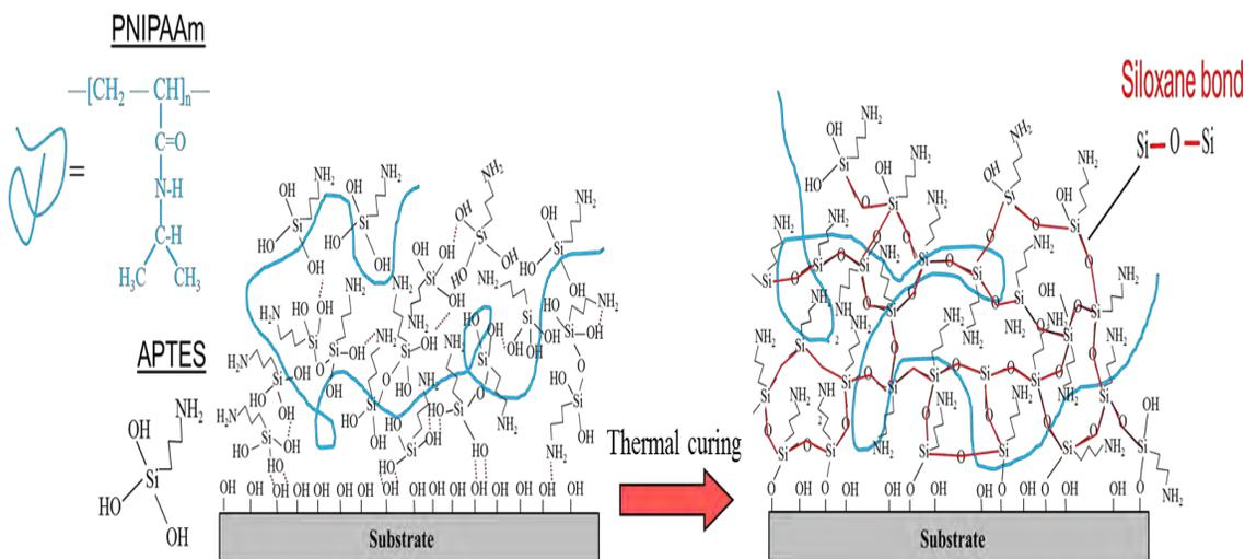
Figure 1.1 pNIPAAm immobilization via the siloxane network (Si-O-Si, shown in red) formed by APTES after thermal curing at 160 °C. The blue line represents the pNIPAAm chain and the dotted red line represents hydrogen bonding. Upon heating, the hydrogen bonds that are formed between the silanol groups (Si-OH) convert to the much stronger covalent siloxane bonds (Si-O-Si), hence forming the cross-linked network.
