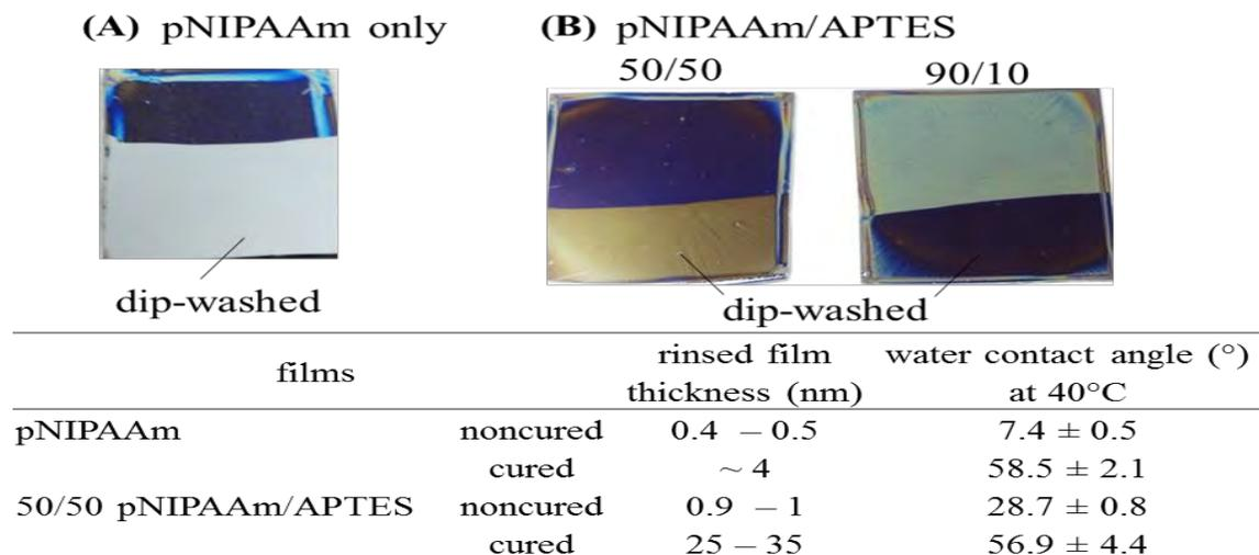
Figure 4.1 The appearance of the 3-days cured films after dip-washing in DI water. (A) pNIPAAm only and (B) 50/50 and 90/10 pNIPAAm/APTES by weight. For imaging purposes (to have better contrast in color), some films were prepared using a higher solute concentration (2 or 3 wt.%) as opposed to 1.5wt.% used in this study. The accompanying table shows the thickness values and water contact angles of the rinsed films prepared using 1.5 wt.% solutes in ethanol.
