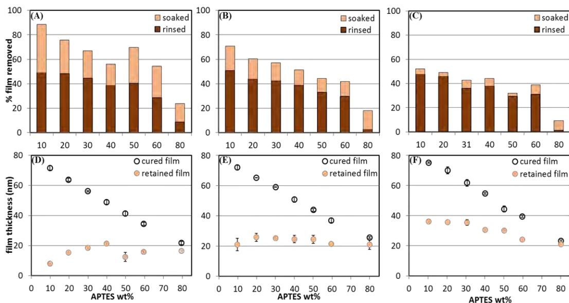
Figure 4.2 % film removal (upper row) and film thickness (lower row) before/after rinsing and further soaking for 3 days in cold water ( $\sim 23$  °C) for films prepared using different pNIPAAm/APTES ratios and cured at 160 °C for 1 day (A & D), 2 days (B&E) and 3 days (C&F).
