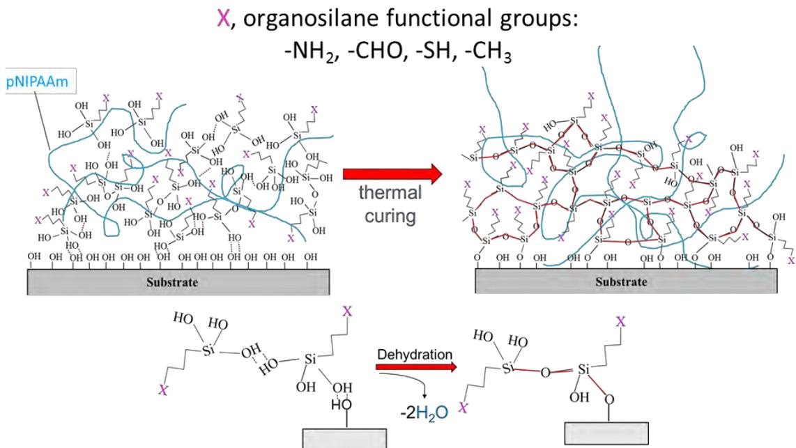
Figure 2.3 Schematic illustration of the siloxane network formation by organosilanes upon thermal curing and subsequent dehydration of the silanol groups (Si-OH) to form siloxane (Si-O-Si, shown in red) bonds.
