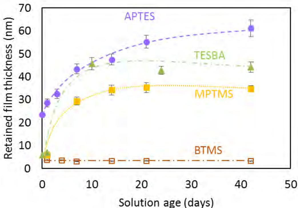
Figure 4.11 The retained film thickness after 3-days soaking for 1.5wt.% 50/50 pNIPAAm/organosilane spin-coated using blend solutions with various ages.
