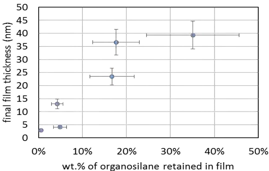
Figure 4.8 The final film thickness after 3 days soaking in water (23 °C) for films prepared using 2 wt.% pNIPAAm/organosilane solution in ethanol.
