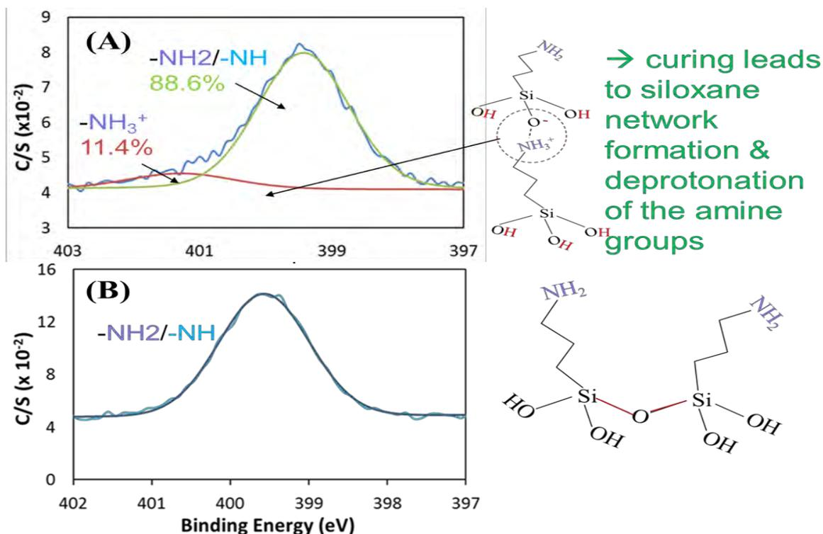
Figure 4.3 High resolution N1s scan showing (A) uncured 50/50 pNIPAAm/APTES and (B) cured 50/50 pNIPAAm/APTES.
