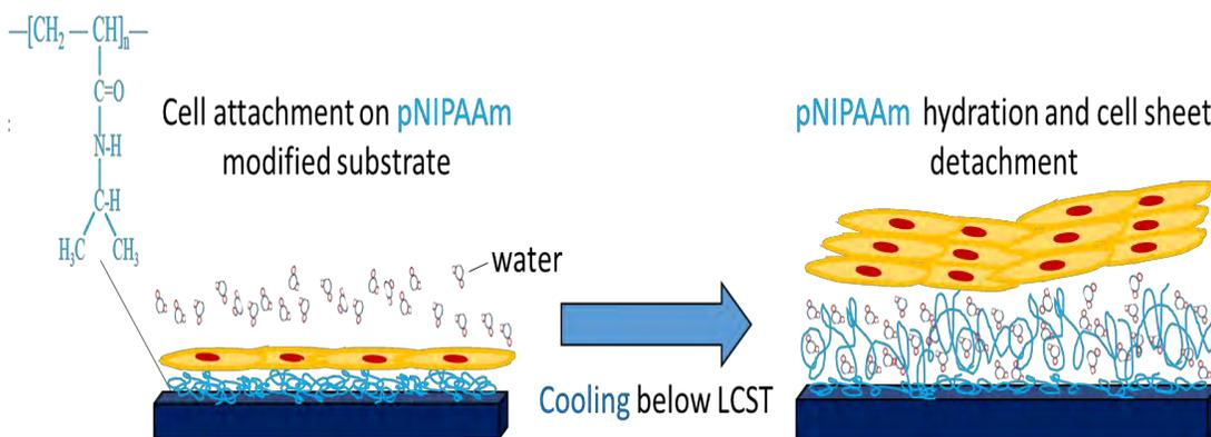
Figure 2.2 Schematic illustration of cell sheet detachment from pNIPAAm-modified surface. Above the LCST, pNIPAAm chains are collapsed and slightly hydrophobic. Below the LCST, pNIPAAm chains are hydrated mediating the cell sheet detachment.
