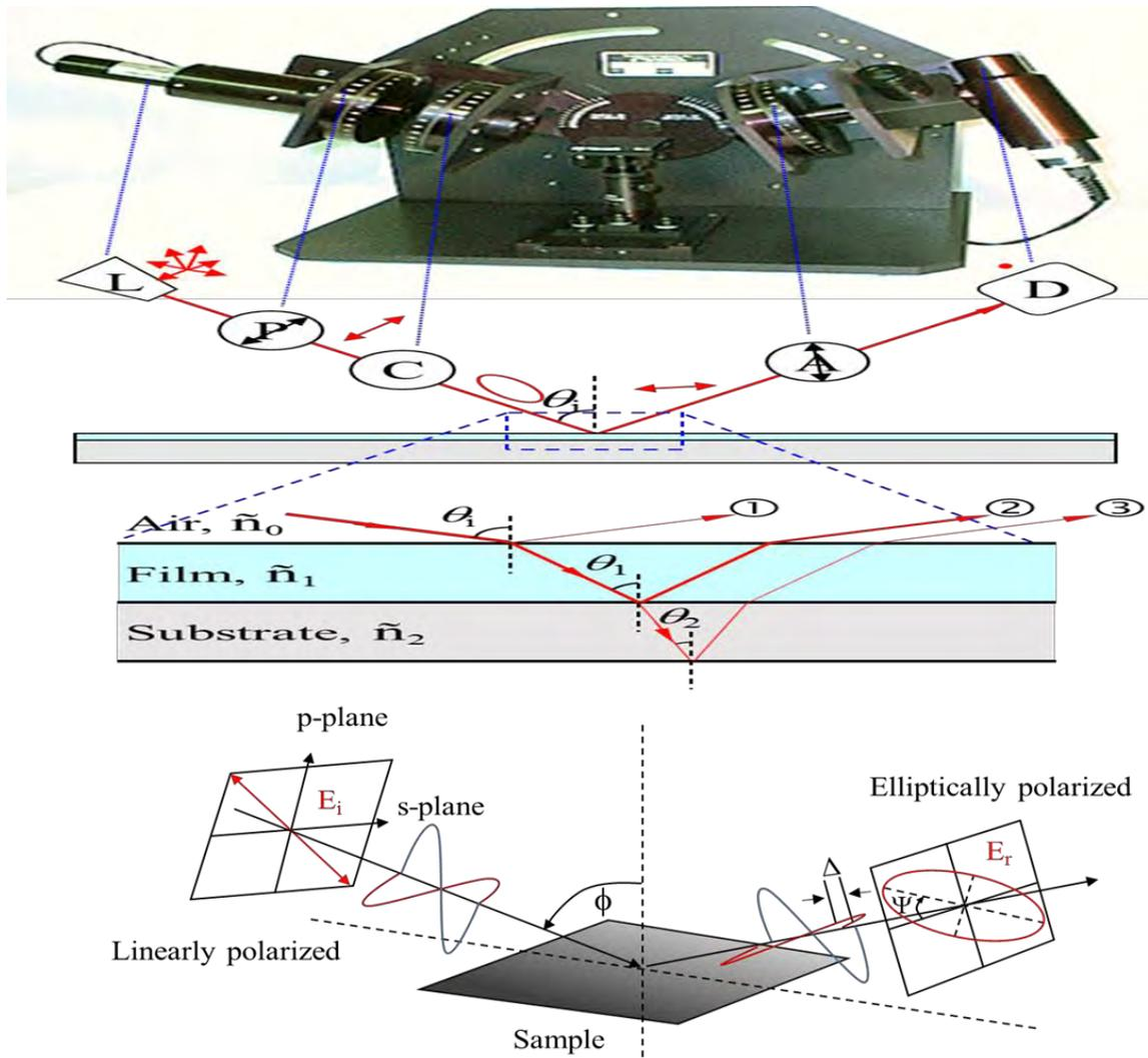
Figure 2.6 A manual ellipsometer along with schematic illustrations of the polarization processes. The analyzer and polarizer values are used to determine the relative amplitude change ( $\Psi$ ) and relative phase change ( $\Delta$ ), respectively, of the laser passes through a film and reflects from the film surface as shown, respectively, as ② and ① in the sketch above.
