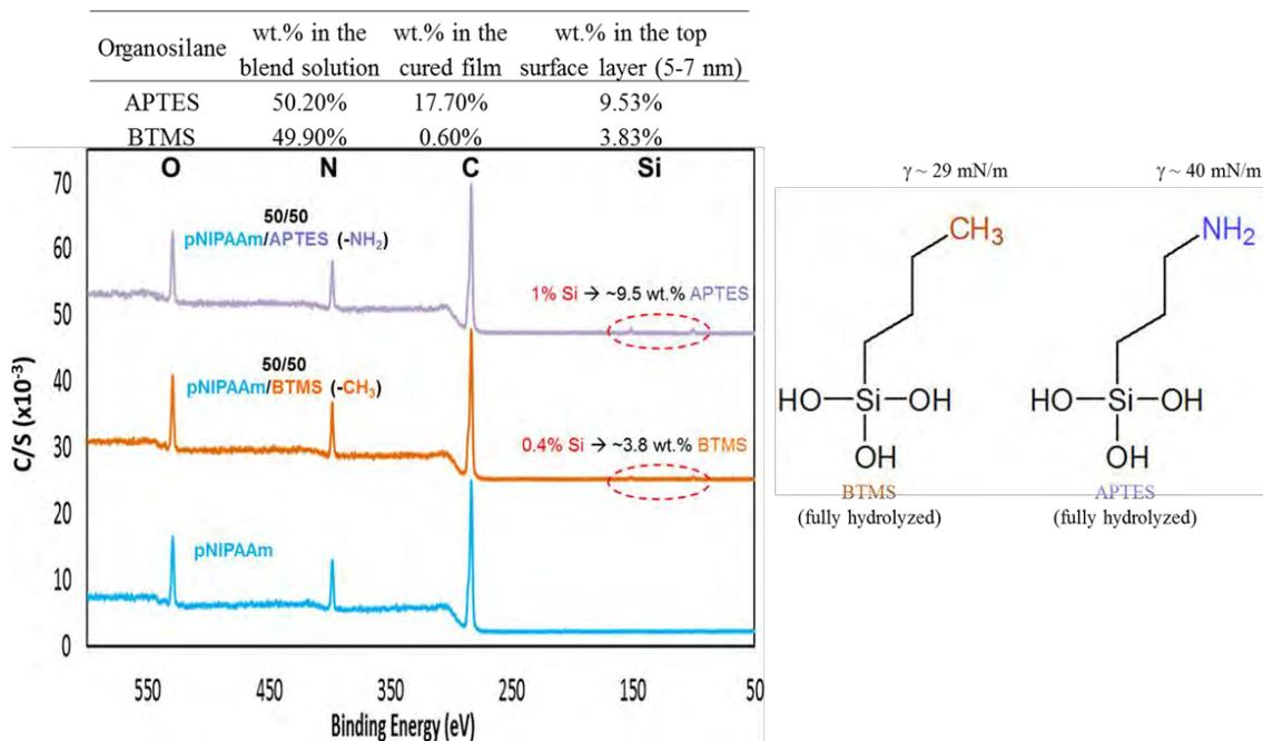
Figure 4.6 XPS survey scans showing the atomic percent of Si present in the top surface layer (5-7 nm) of cured non-rinsed 50/50 pNIPAAm/BTMS or APTES. The accompanying table shows the total wt.% of the organosilane in the original solution, in the cured film and in the top surface layer of the films. The chemical structure of fully hydrolyzed BTMS and APTES is shown on the right along with their surface tension values.
