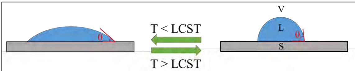
Figure 2.7 A schematic illustration showing the reduction in contact angle ( $\theta$ ) when the temperature is lowered below the LCST.
