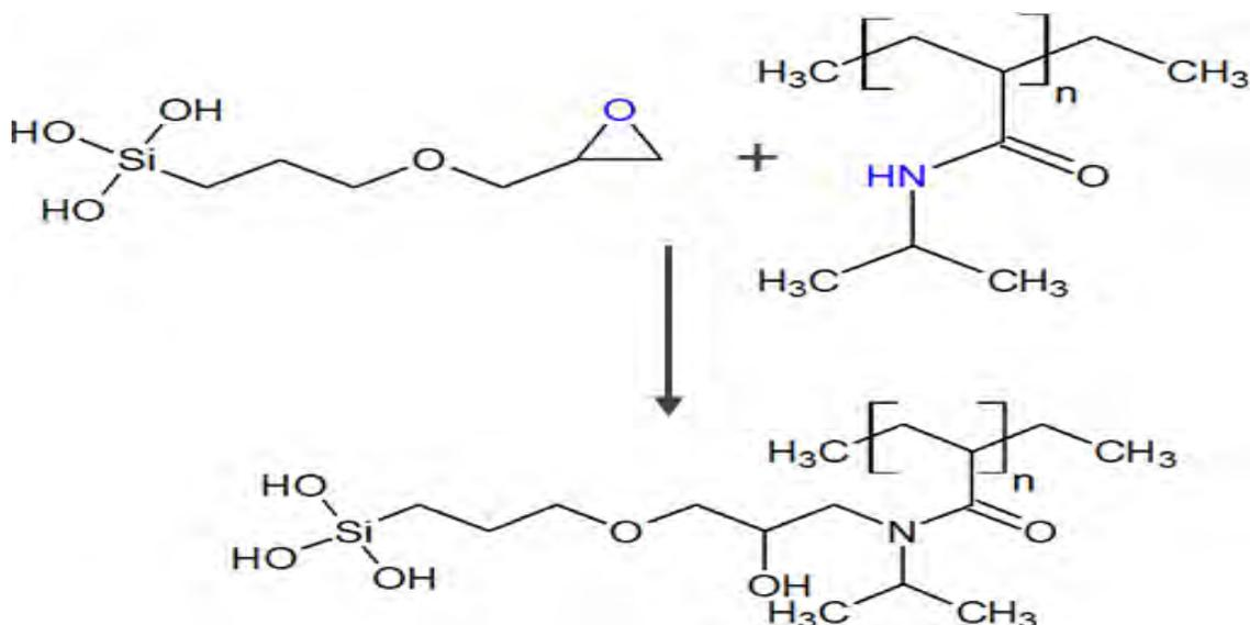
Figure 2.4 A schematic illustration of the possible reaction between the epoxy group in EPPTMS and the secondary amine group in pNIPAAm. The silanol (Si-OH) groups can then react with the substrate resulting in the chemical grafting of pNIPAAm to the substrate.
