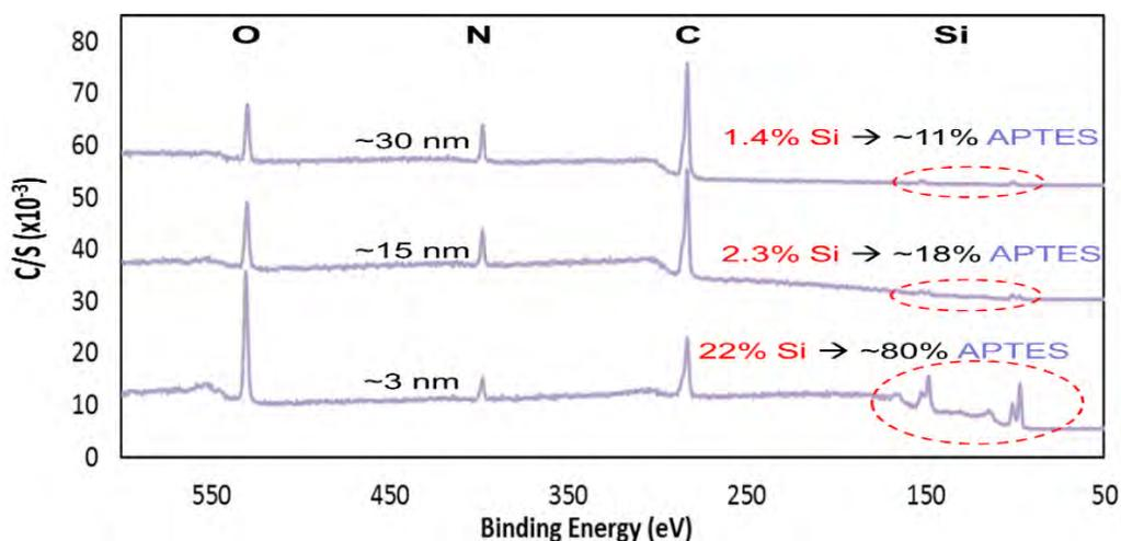
Figure 4.4 XPS survey scans showing the Si atomic percent for 50/50 pNIPAAm/APTES films etched to different thicknesses. The mol.% APTES shown is estimated from the atomic % of Si assuming that the APTES molecule is fully hydrolyzed. The silica layer on the silicon wafer has a thickness of 2.5 nm, and the average X-ray penetration depth of 6 nm was used for the estimation.
