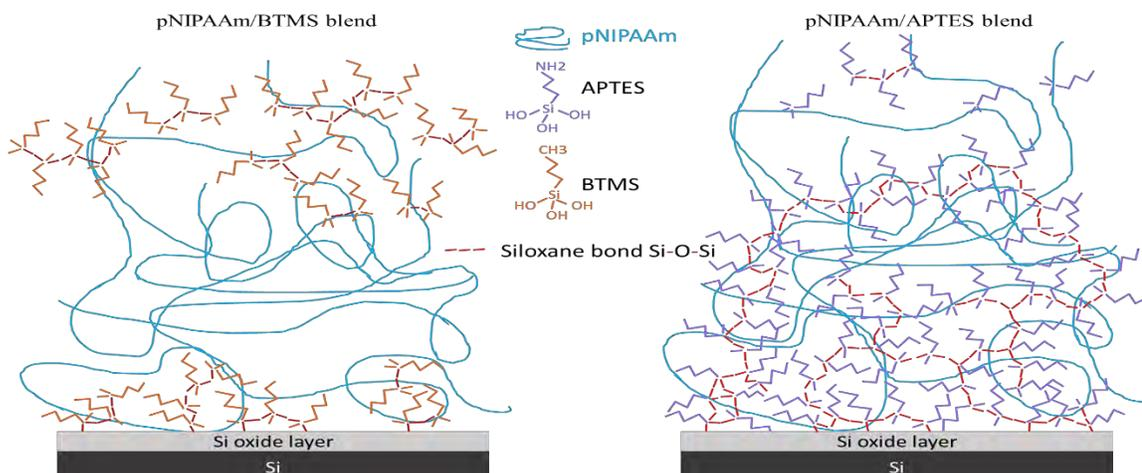
Figure 4.7 A schematic illustration of the network formed by BTMS (left) and APTES (right) after curing.
