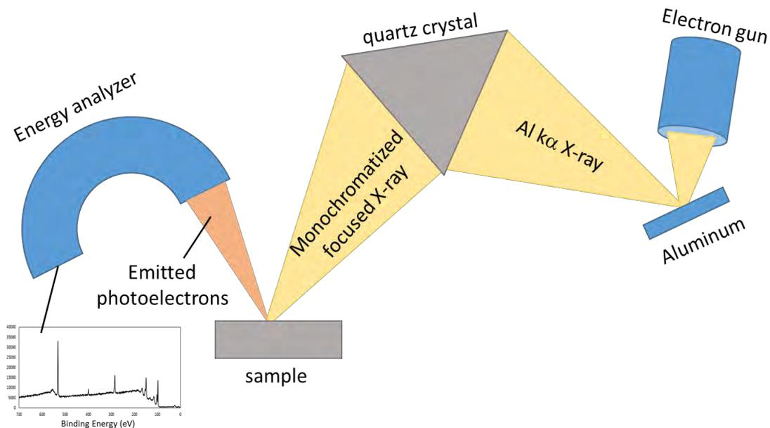
Figure 2.5 Schematic illustration of the XPS spectrum generation process
