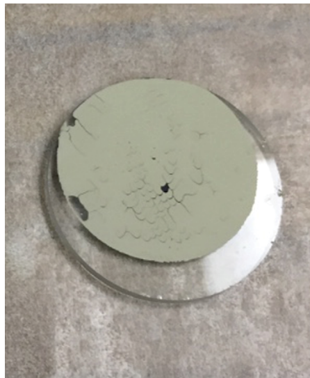
Figure 2.6. Photographs of X-ray Diffraction instrument and supplies. A) XRD instrument used for sample analysis. B) Sample holder for bulk XRD measurements. B) Glass slides used for mounting the clay fraction.
