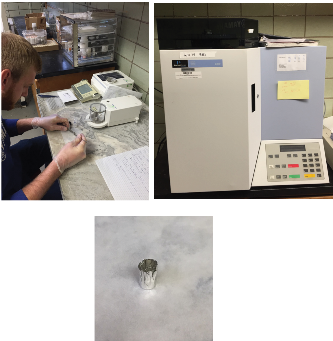
Figure 2.13. Photographs of CHN analyzer, supplies, and preparation. Top left photo taken by Annie Hartwell.
