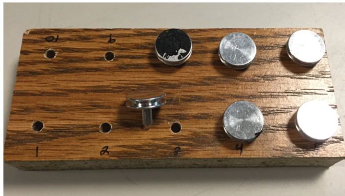
Figure 2.12. Photographs of the ESEM and supplies. A) ESEM. B) Sample holders and adhesive used to mount samples.
