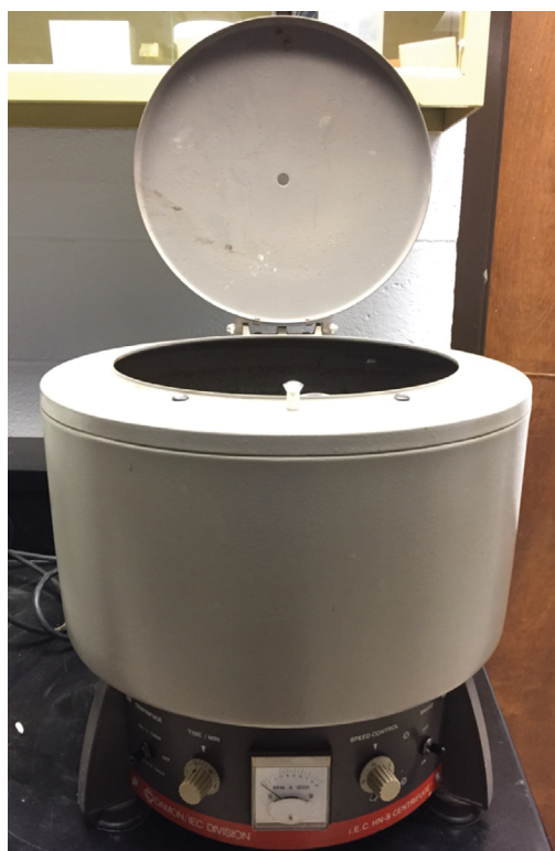
Figure 2.7. Photograph of equipment used for extraction of the clay sized fraction. (A) Centrifuge used for separating the <2\ \mu\text{m} fraction and (B) the equipment used to vacuum the clay minerals onto the cellulose filters.
