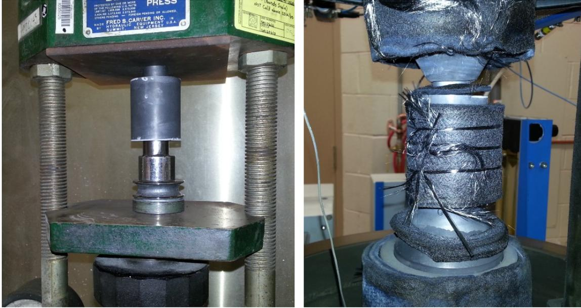
Figure 6.3: Powder being pressed in graphite dies: cold pressed die (Left) and die mounted with insulation for SPS run (Right).
