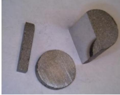
Figure 9.8: Typical hot pressed skutterudite ingots, 1/2" diameter by 1" tall. Shown cut for electrical measurement (rectangular prism) and thermal measurement (disk).
