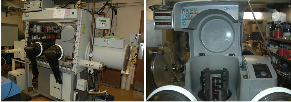
Figure 6.2: Picture of the MBRAUN glovebox (Left) and PM100 planetary mill (Right) used for this study.
