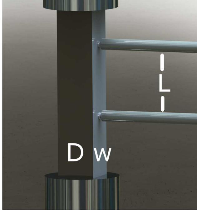
Figure 7.1: Potentiometric configuration for Seebeck coefficient or electrical resistivity measurement. Samples cut to the shape of a rectangular prism or cylinder are held in place by electrodes, top and bottom, while two probe thermocouples make contact on a single face of the sample.
