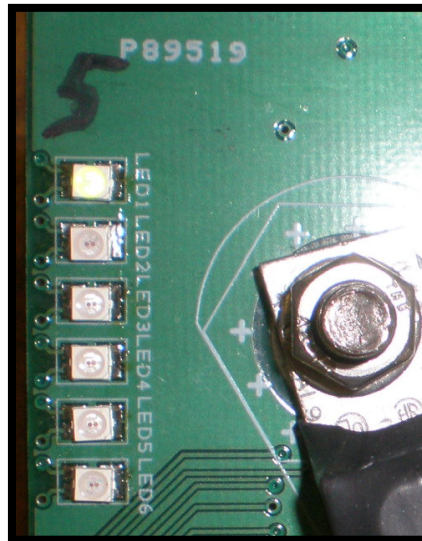
Figure 5.18: Actual Implementation of dual color LEDs.
