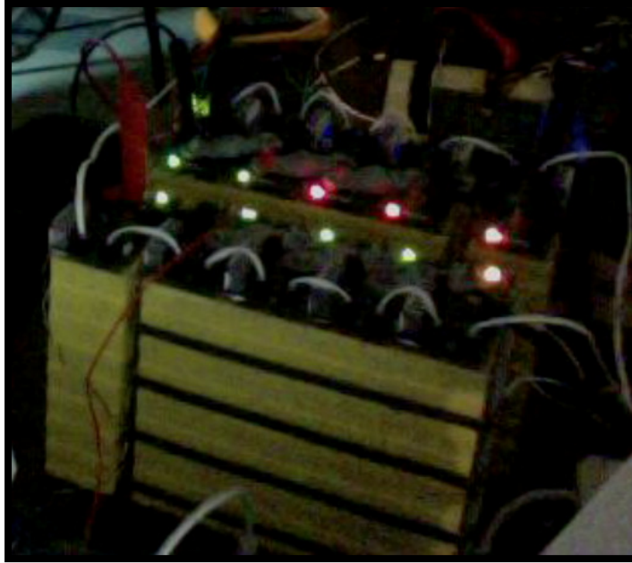
Figure 7.4: Battery Pack with ICMU and ICMU/BPMU Hybrid attached to each cell. As pictured here, 4 cells are bypassing current since they have reached a voltage of at least 3.8V.
