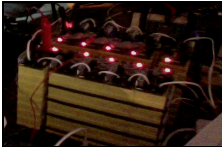
Figure 7.6: Battery Pack with ICMU and ICMU/BPMU Hybrid attached to each cell. As pictured here, all cells are in bypass. Shortly after this picture was taken, the BPMU commanded the Charger to discontinue the charging process.
