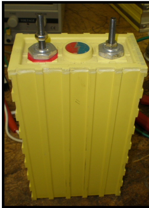
Figure 5.1: Single 60Ah LiFePO 4 Cell.
