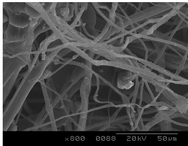
Figure 9.10: SEM image of an untested N100 respirator fibers
