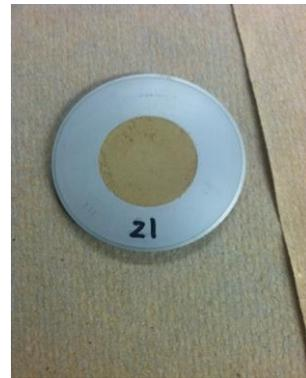
Figure 14 Packed XRD powder sample
