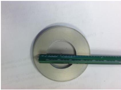
Figure 13 Metal XRD powder sample holder.
