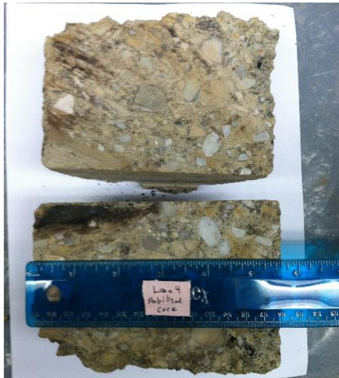
Figure 15 Inside Surface of Loc 4 Stabilized Core Inspected for White Precipitate.
