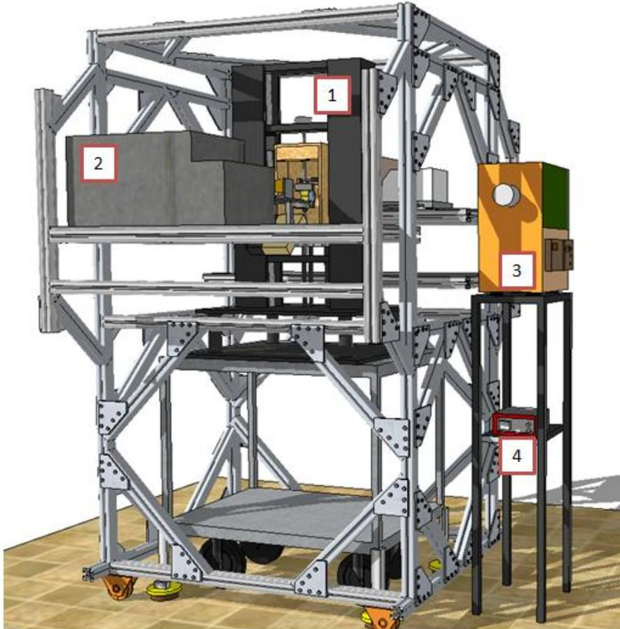
Figure IV-1 Real-time rheo-optical measurement platform. 1) Inner layer is a custom-built uniaxial stretching machine. 2) The outer layer is a custom build URS-FT-IR spectrometer. 3) Hot air blower. 4) Visible wavelength spectrometer.
