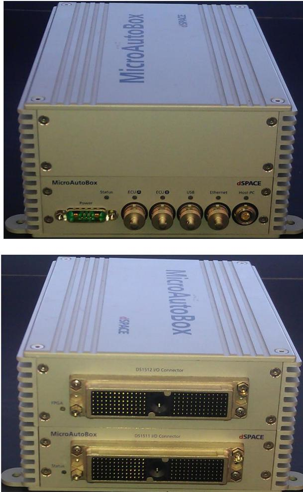
Figure 6-1: dSPACE MicroAutobox II, Front and rear view.
