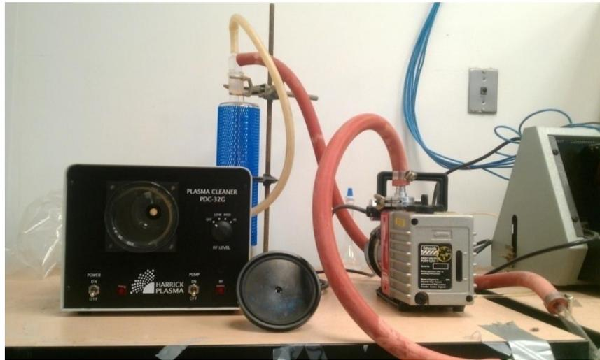
Figure 4-6 Plasma cleaner PDC- 32G equipped with vacuum pump
