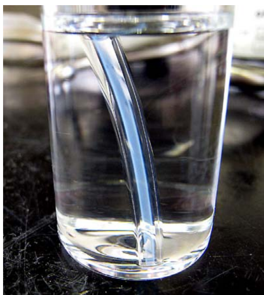
Figure 4.26. Picture of PVC-g-PHEMA tube in THF. The inside of the tube appears white because the PHEMA that is grafted to the interior chains is not soluble in THF.
