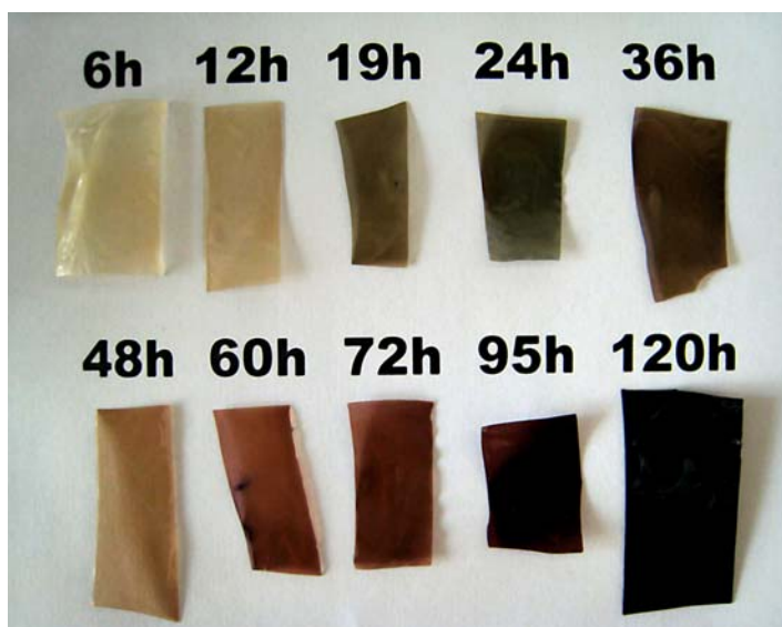
Figure 4.40. Image of PVC-g-P4VP films quaternized with 1-bromohexane in ethyl acetate at 80 °C for various reaction times.
