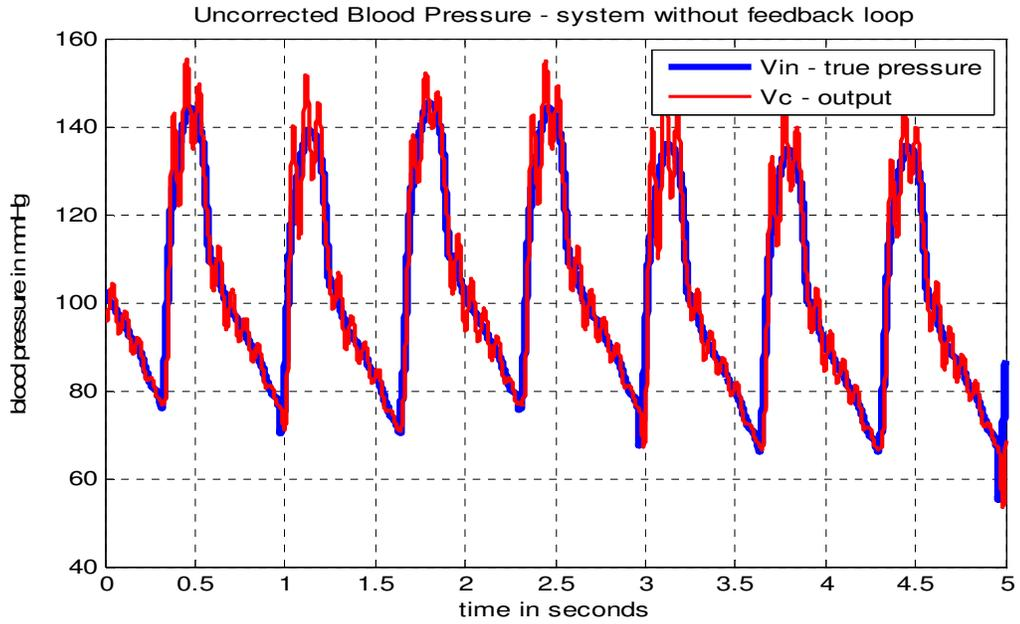
Figure 5.3: True blood pressure wave and output pressure wave for – bubble size: 15uL and bubble location  $l = 0.9\text{m}$  (refer table 4.1)
