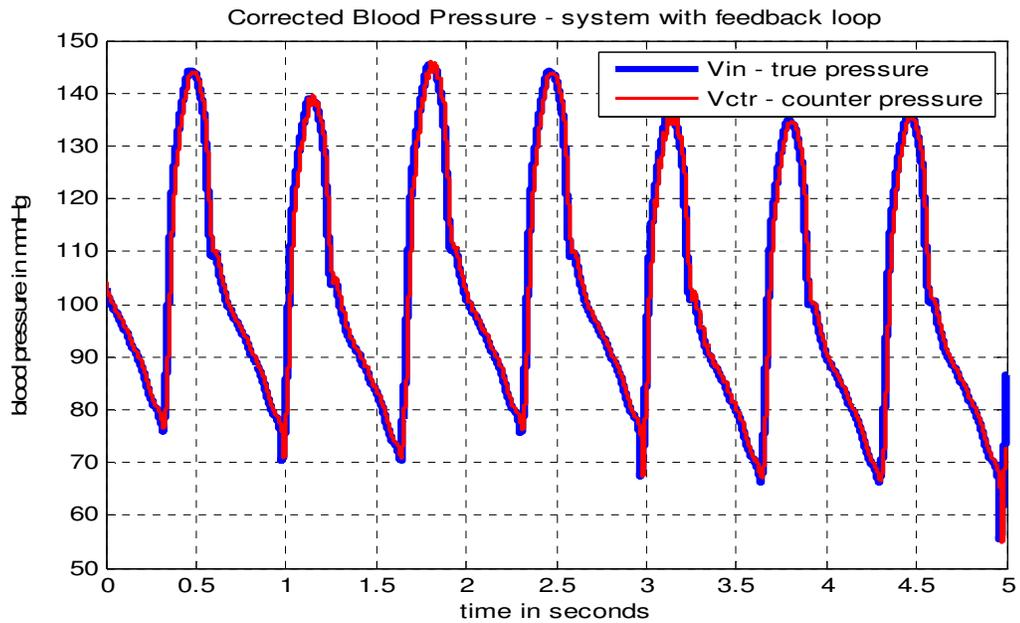
Figure 5.10: True blood pressure wave and counter pressure wave for – bubble size: 20uL and bubble location  $l = 0.6m$  (refer table 4.1)
