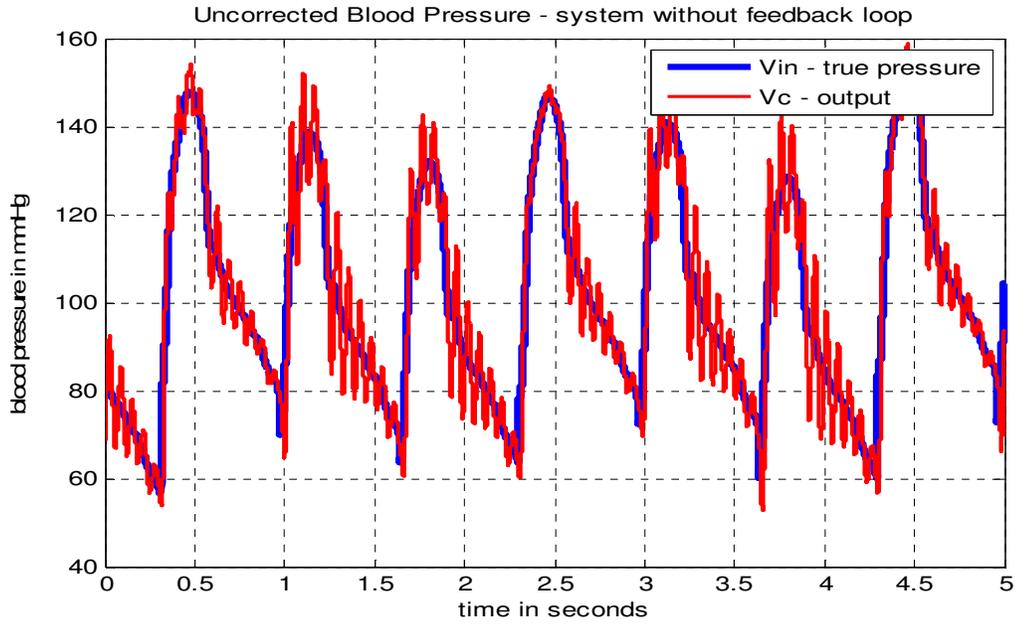
Figure 5.13: True blood pressure wave and output pressure wave for – bubble size: 5 $\mu$ L and bubble location  $l = 1.2$ m (refer table 4.1)
