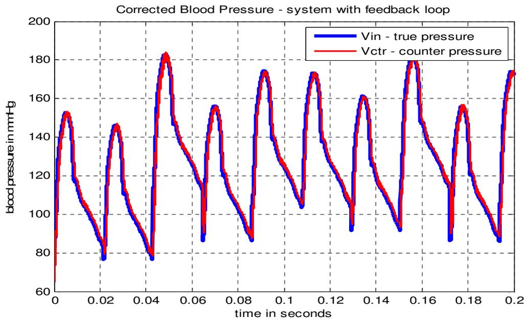
Figure 5.8: True blood pressure wave and counter pressure wave (output of the feedback loop) for a system with feedback gain of 100
