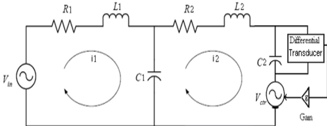
Figure 3.7 Feedback loop used to determine the required counter pressure
