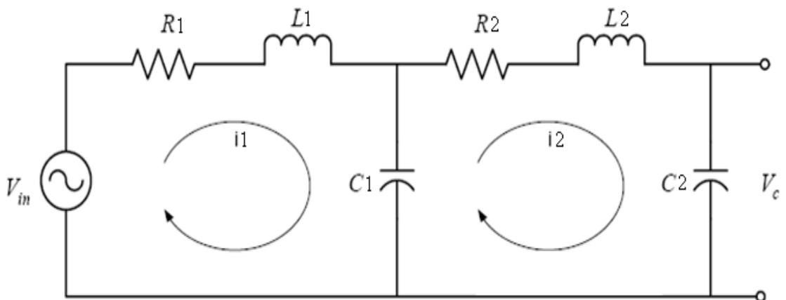
Figure 3.5: Catheter transducer system as a fourth order dynamic system
