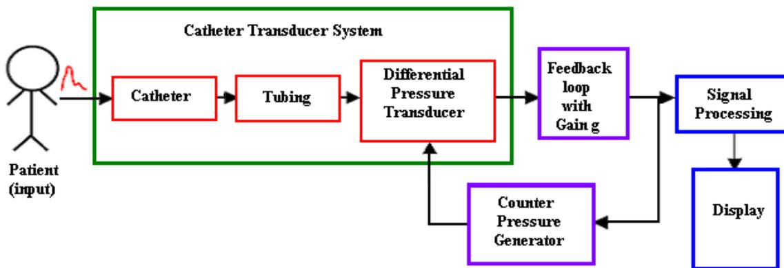
Figure 6.1: Future vision - Implementation of counter pressure on an actual catheter transducer system [1]
