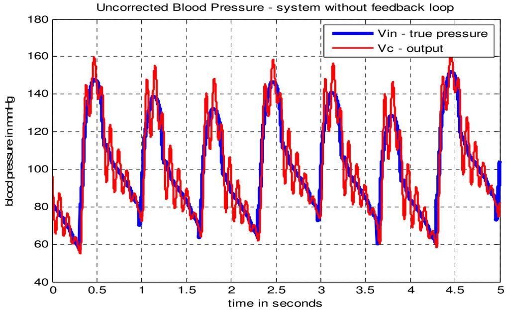
Figure 5.5: True blood pressure wave and output pressure wave for – bubble size: 20uL and bubble location  $l = 0.6m$  (refer table 4.1)
