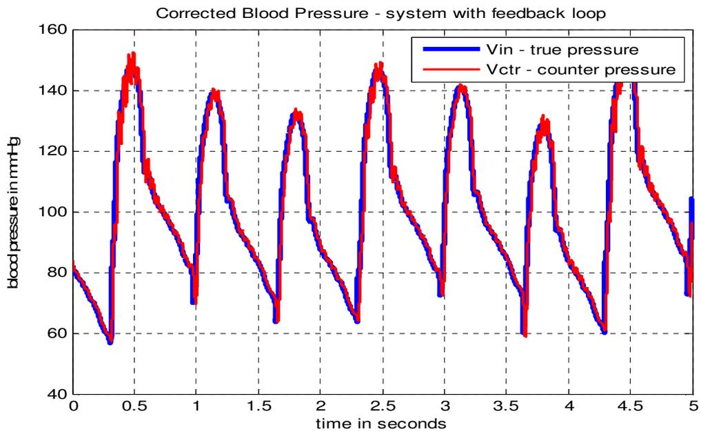
Figure 5.14: True blood pressure wave and counter pressure wave for – bubble size: 5 $\mu$ L and bubble location  $l = 1.2$ m (refer table 4.1)
