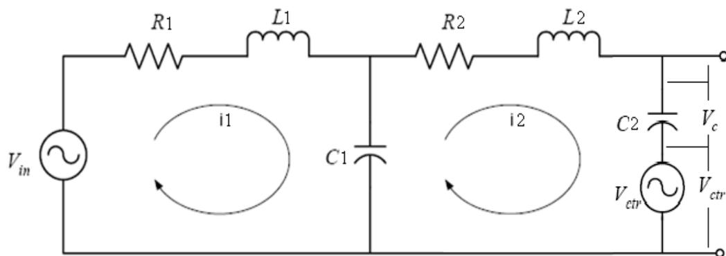
Figure 3.6: Catheter transducer system as fourth order dynamic system with counter pressure source
