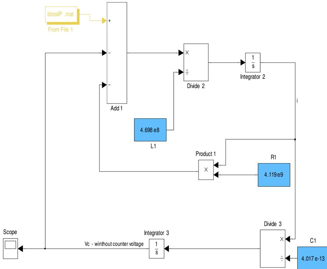
Figure 4.2: MATLAB Simulink model of catheter transducer system without the counter pressure source
