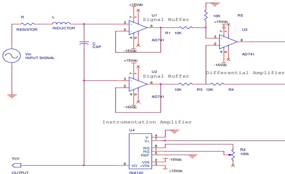
Figure 4.4: Schematic of the electrical circuit (2<sup>nd</sup> order system), equivalent to the catheter transducer system with a counter pressure source
