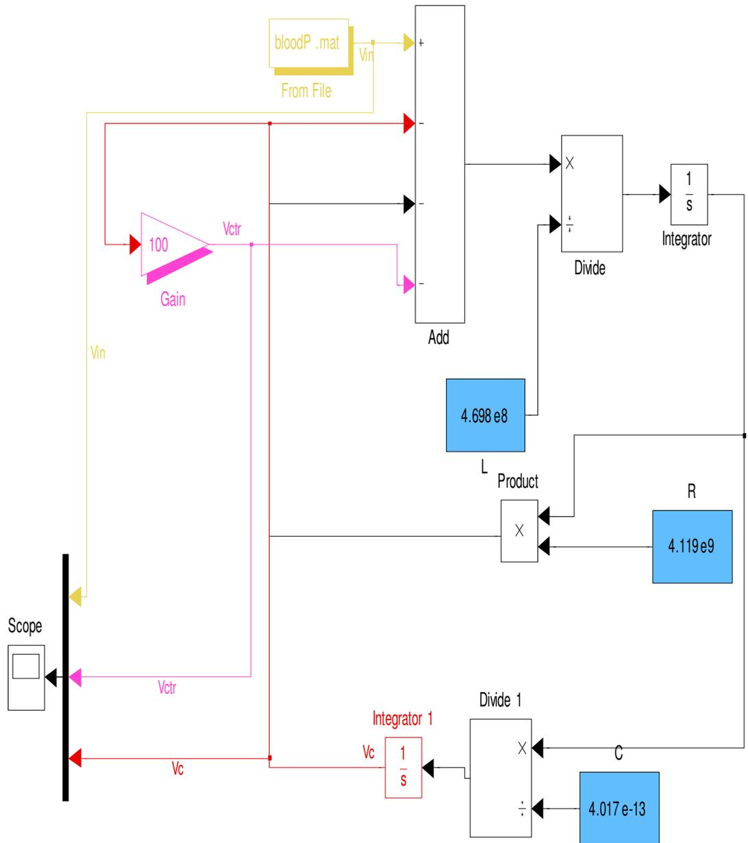
Figure 4.1: MATLAB Simulink model of catheter transducer system with feedback loop (Second order dynamic system)
