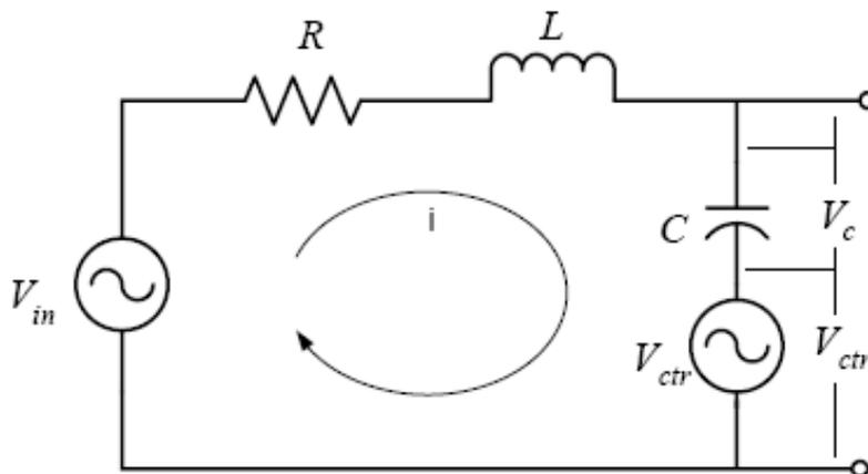
Figure 3.2: A counter voltage source added to the electrical circuit
