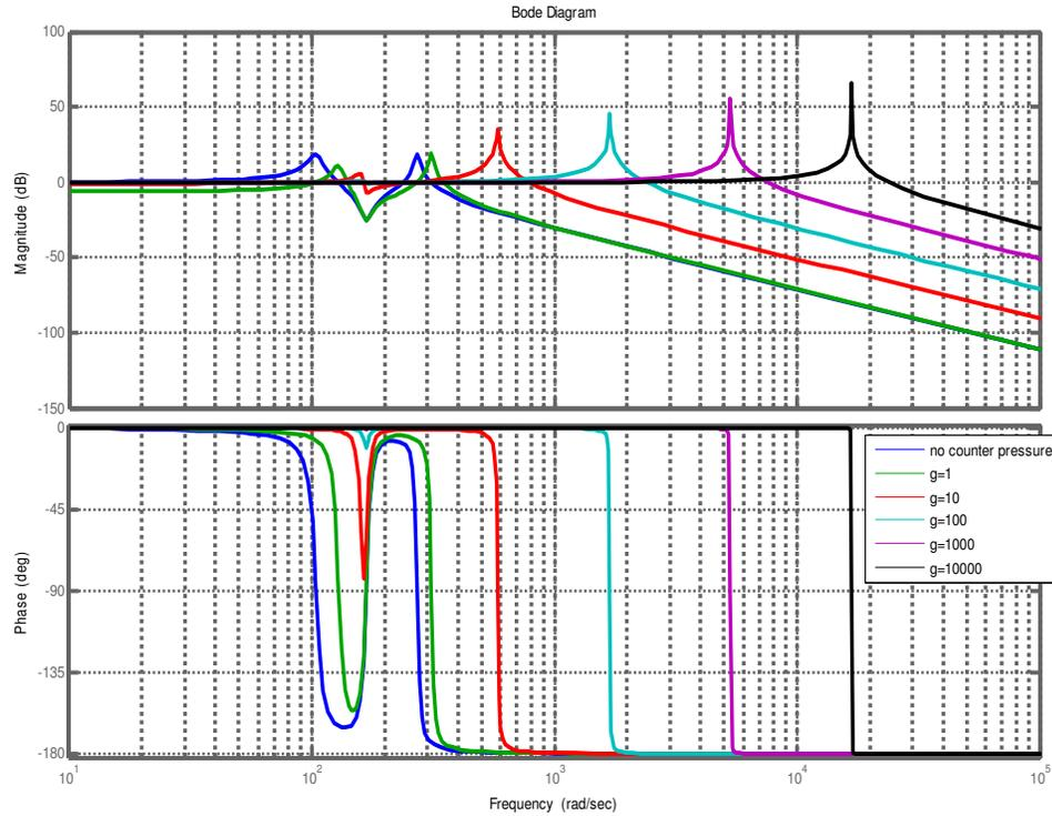
Figure 3.8: Frequency response of the system with and without counter pressure source. Parameters used (bubble location 1 = 0.9m and bubble size 25uL) [1]:  $R = 1.5445 \times 10^9 \text{kg/m}^4\text{s}$ ,  $L = 1.7615 \times 10^8 \text{kg/m}^4$ ,  $C = 2.0085 \times 10^{-13} \text{m}^3/\text{Pa}$
