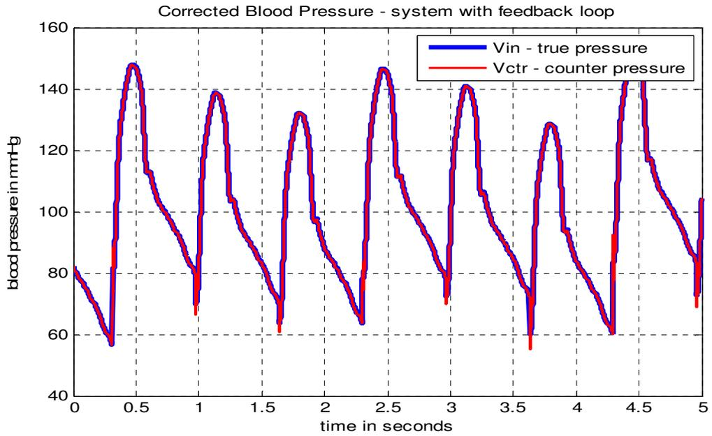
Figure 5.6: True blood pressure wave and counter pressure wave for – bubble size: 20uL and bubble location  $l = 0.6m$  (refer table 4.1)
