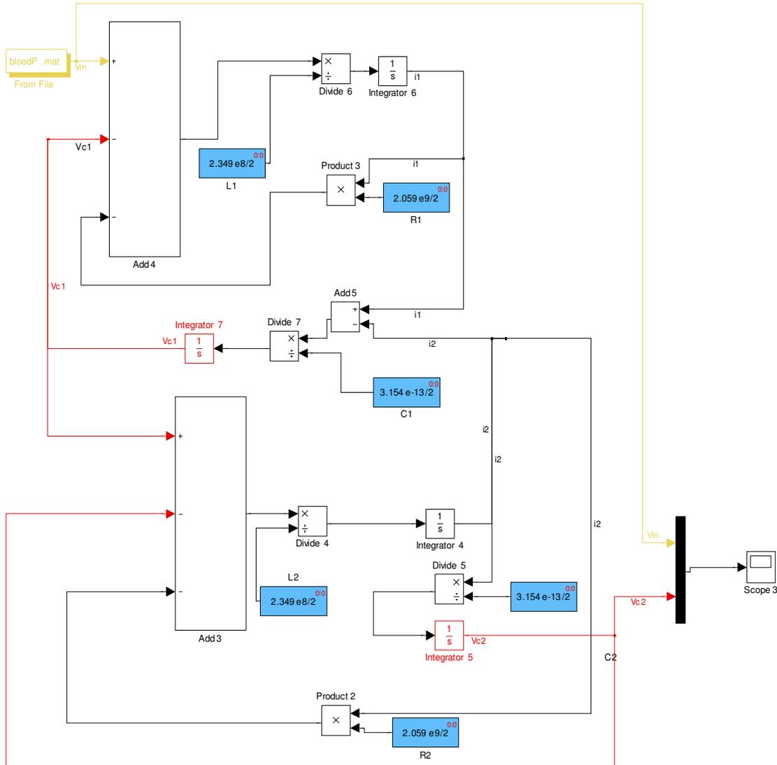
Figure 4.8: MATLAB Simulink model of catheter transducer system without the counter pressure source
