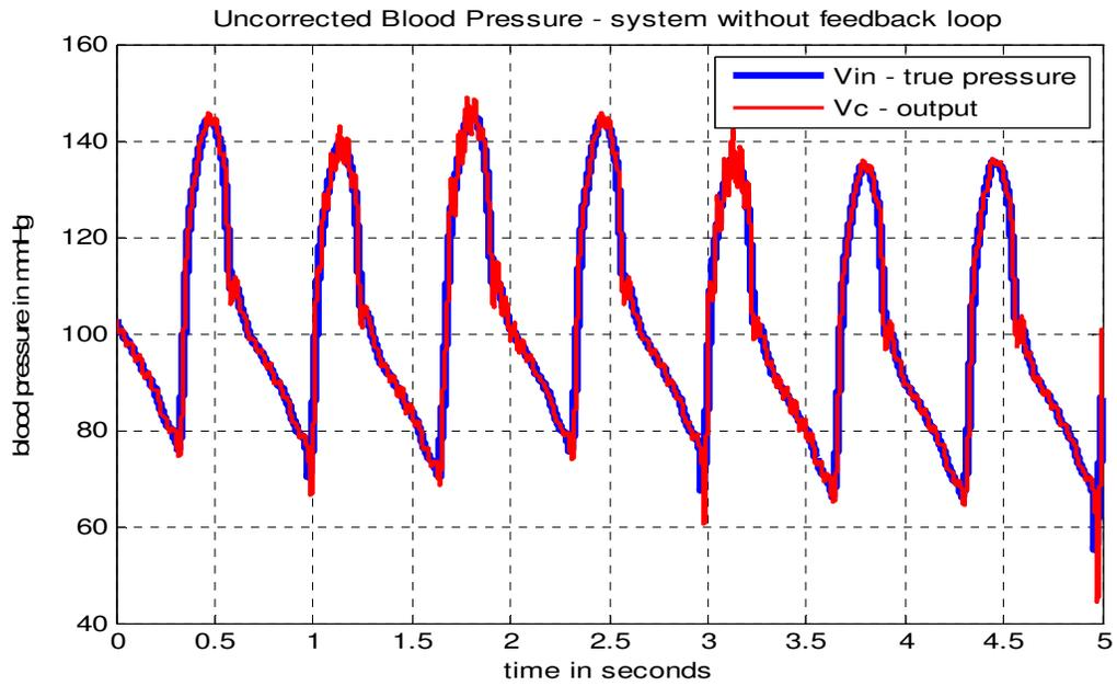
Figure 5.9: True blood pressure wave and output pressure wave for – bubble size: 20uL and bubble location  $l = 0.6m$  (refer table 4.1)
