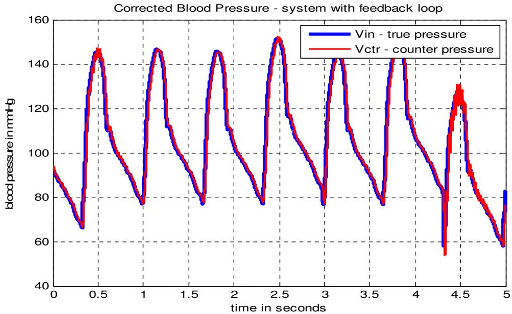
Figure 5.12: True blood pressure wave and counter pressure wave for – bubble size: 5uL and bubble location  $l = 0.9\text{m}$  (refer table 4.1)
