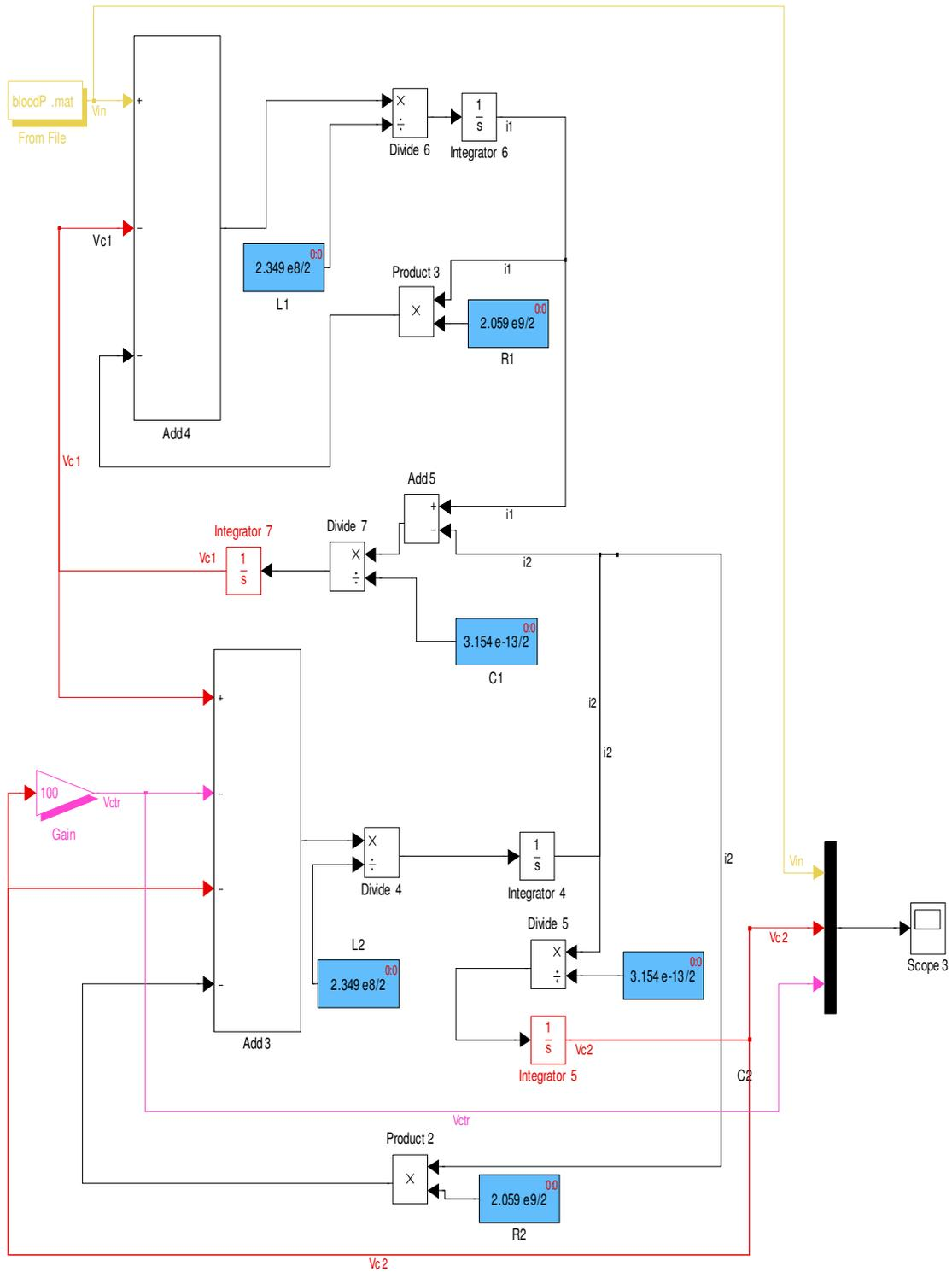
Figure 4.7: MATLAB Simulink model of catheter transducer system with feedback loop (counter pressure source)
