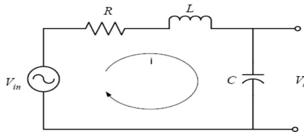
Figure 3.1: Electrical circuit (2<sup>nd</sup> order system) of the catheter-transducer system
