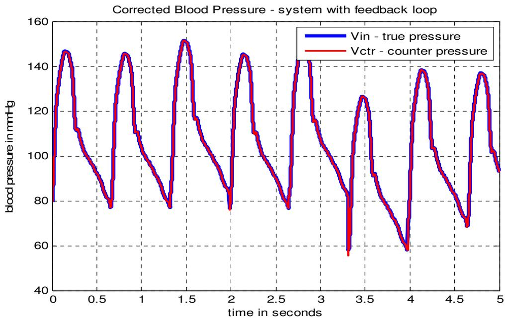
Figure 5.2: True blood pressure wave and counter pressure wave for – bubble size: 5 $\mu$ L and bubble location  $l = 1.2$ m (refer table 4.1)
