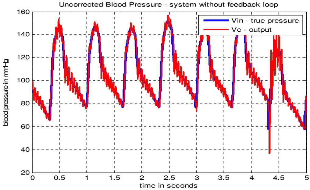
Figure 5.11: True blood pressure wave and output pressure wave for – bubble size: 5uL and bubble location  $l = 0.9\text{m}$  (refer table 4.1)
