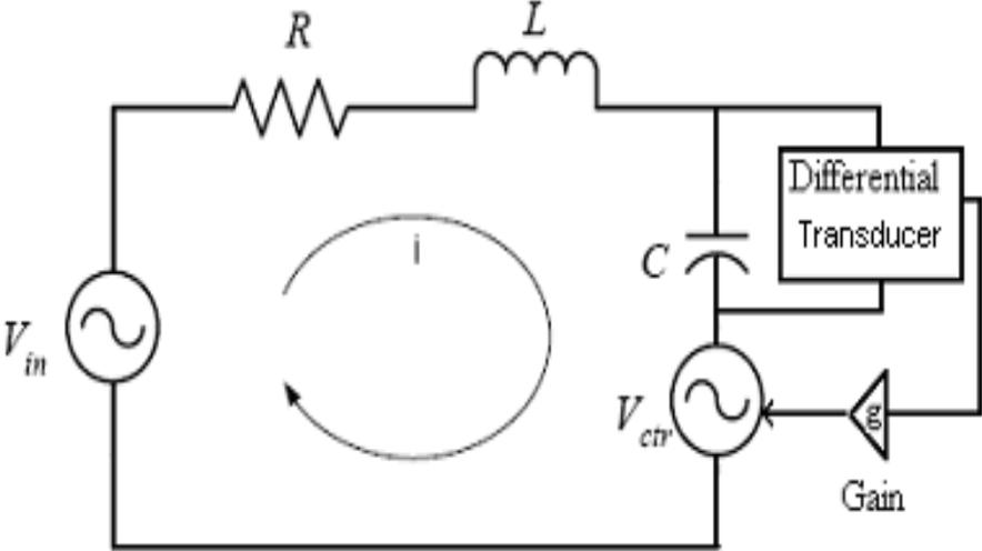
Figure 3.3: Feedback loop used to determine the required counter pressure
