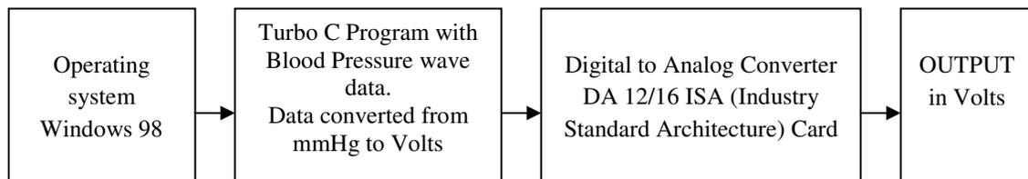
Figure 4.5: Generating blood pressure signal using a computer
