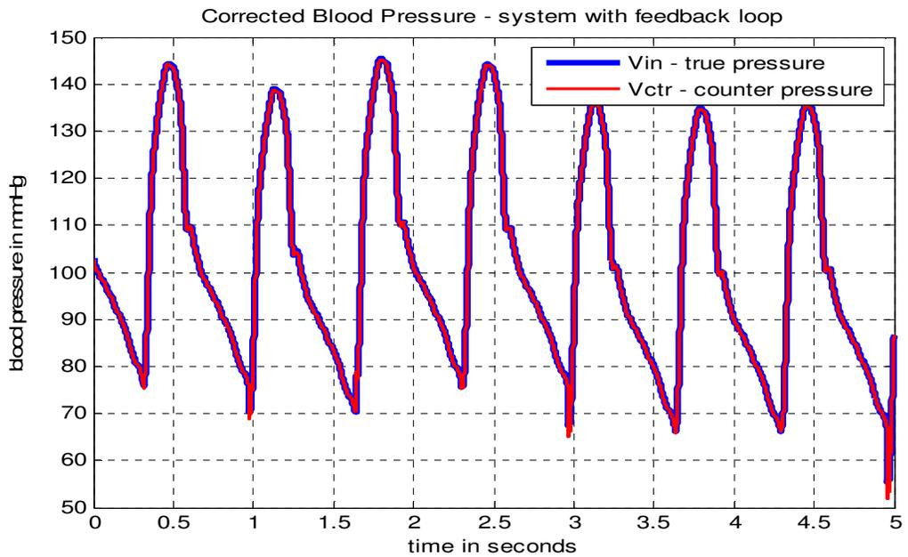
Figure 5.4: True blood pressure wave and counter pressure wave for – bubble size: 15uL and bubble location  $l = 0.9\text{m}$  (refer table 4.1)
