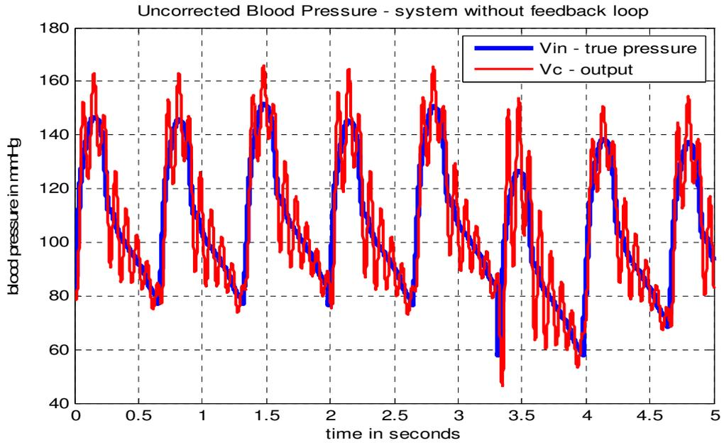
Figure 5.1: True blood pressure wave and output pressure wave for – bubble size: 5 $\mu$ L and bubble location  $l = 1.2$ m (refer table 4.1)
