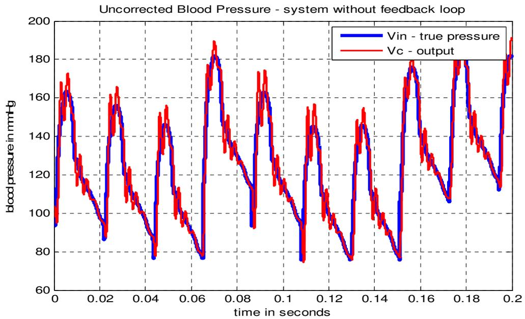
Figure 5.7: True blood pressure wave and output pressure wave for a system without counter pressure
