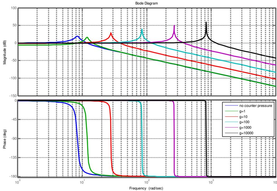
Figure 3.4: Frequency response of the system with and without counter pressure source. Parameters used (bubble location  $l = 0.9\text{m}$  and bubble size  $25\mu\text{L}$ ) [1]:  $R = 3.089 \times 10^9 \text{ kg/m}^4\text{s}$ ,  $L = 3.523 \times 10^8 \text{ kg/m}^4$ ,  $C = 4.017 \times 10^{-13} \text{ m}^3/\text{Pa}$
