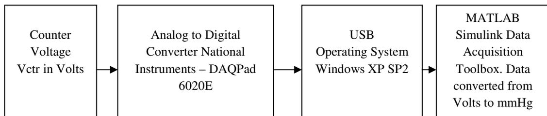
Figure 4.6: Data Acquisition setup
