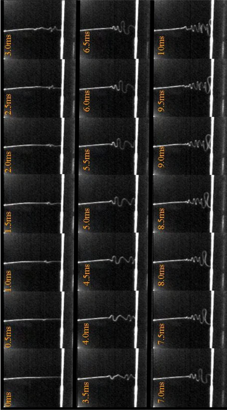
Figure 3.7 High frame rate camera images of the onset and development of the electrical bending instability along an electrically driven jet. The time at which the voltage was lowered is shown in the upper left corner.
