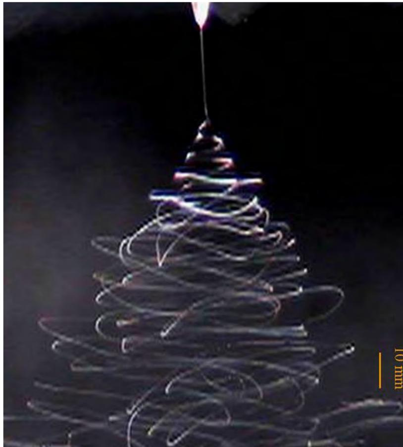
Figure 3.1 Electrospinning jet with electrical bending instability
