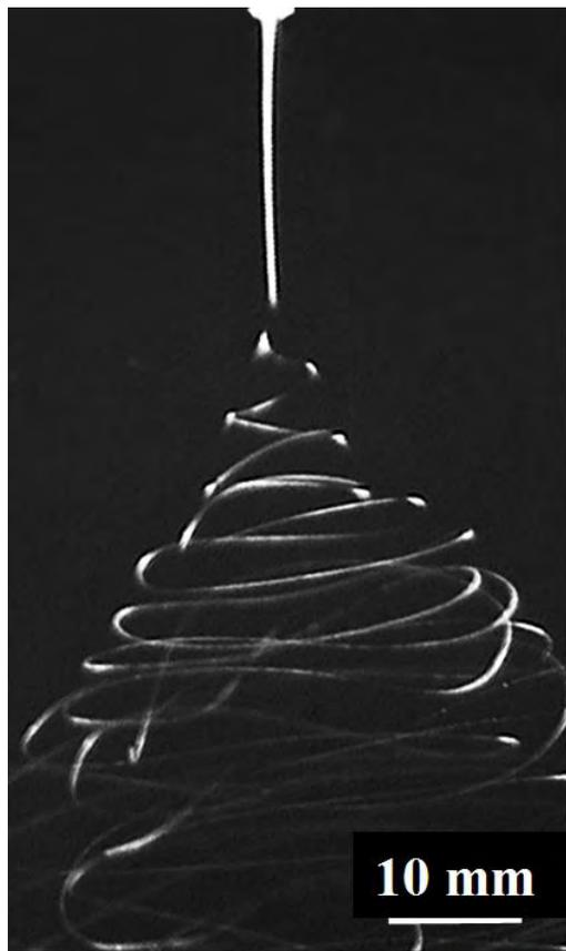
Figure 5.3. Electrospinning jet with electrical bending instability
