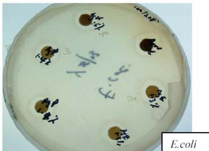
Figure 1-6. Kirby-Bauer diffusion method compared on E-coli for 6a compared to \text{AgNO}_3 . 39
