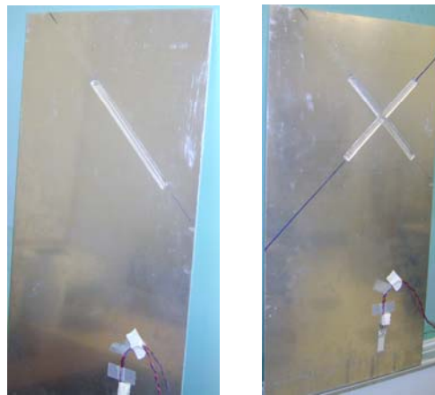
Figure 3.9 Final Damages D1 (left) and D2
