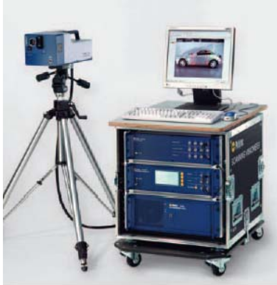
Figure 3.2 Scanning Laser Vibrometer (Laser Head on tripod and computer screen on the top of controller)
