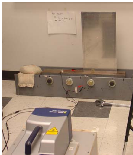
Figure 3.7 SLV Laser Head and Specimen after the fixed Scan Head Optimal Distance
